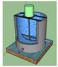
Schematic of Lime treatment drum system
