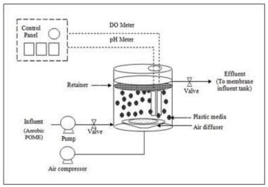
Schematic of MBBR & Oxygen blower for Amid to Nitrate conversion
