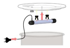
• Step 7: Two pin UV-C tube in plug into solar UPS battery.
