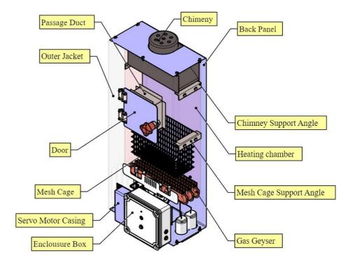
LPG based sanitary pad Incinerator BOM
