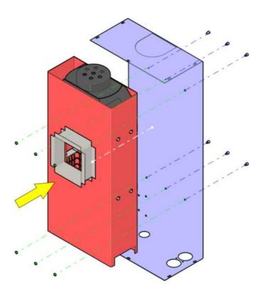
Heating chamber sub-assembly & Back Panel assembled together by matching appropriate holes & joined with fasteners.
