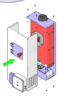
• LPG based sanitary pad incinerator having following subassemblies are Back panel, Heating chamber, Regulated gas geyser system, Outer jacket
