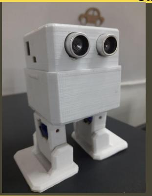
Otto biped robot is an open source robot which you can print on 3d printer and assemble with the given manual and play with codes and to make your robot dance, walk, follow and avoid.
