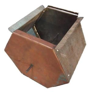
• Take flanges as shown in point number 4. Insert it from both side in a such way that it seats on the central rod.
