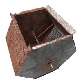
• Take pipe as shown below. Insert it from both side in a such way that it seats on the central rod as well as on the bush.
