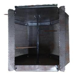
• Note that both baffles must be welded in the same plane but in the opposite sides to each other.
