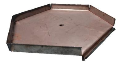
3. Take the Flat punched mesh sheet and bend it from the bending lines (Shown by dotted portion in sketch) to form a hexagon ie) The angle between successive sides will be 120 degrees.
